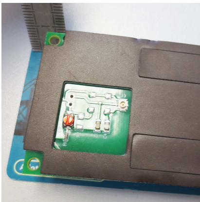
GOOD ≈ 1cm between the antenna and the card
